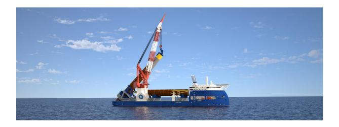
Following feasibility and concept studies in 2023, Penta-Ocean Construction selected Ulstein for the project. Ulstein proposed the HX118 with the U-STERN<sup>™</sup>, a design that builds on Ulstein's successful track record of crane vessels. The selected design offers a well-balanced combination of a flush work deck, lifting capacity, accommodation and DP capability and will be the largest X-BOW<sup>®</sup> vessel to date.
